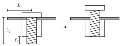
The gray bars represent the wheel spokes which rotate around the central axis and lift the screw. There are eight spokes on the wheel. Let L = 1.5 m,  $\ell_1 = 0.90 \text{ m}$ , and  $\ell_2 = 0.20 \text{ m}$ . Friction is negligible.
