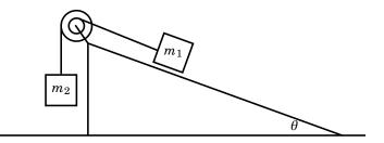
The mass  $m_1$  is attached to a pulley of radius  $R_1$ . This pulley shares an axis with one of radius  $R_2$ , which is subsequently attached to  $m_2$ . We have  $3R_2 = 4R_1$  and  $3m_2 = m_1$ . The mass  $m_2$  is considered the load.
