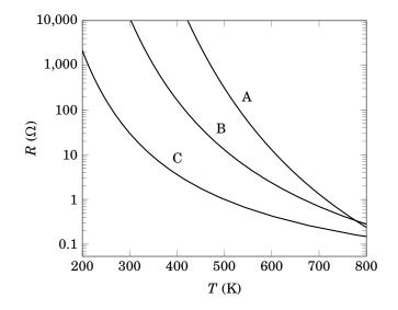
(a) (3 points) Which of the three thermistors would you pick to measure resistances between 200°C and 300°C with a digital ohmmeter? Why? Assume the ohmmeter measures to 3 significant figures.
